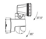
The beam angle of the LED spotlight heads can be adjusted by turning the Lamp Cap Rings around the LED spotlight heads.
