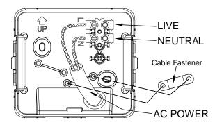
(6) Refit the Spotlight onto the wall box and secure with the two clips. Refit the wall box screw at the base of the unit (if fitted).
